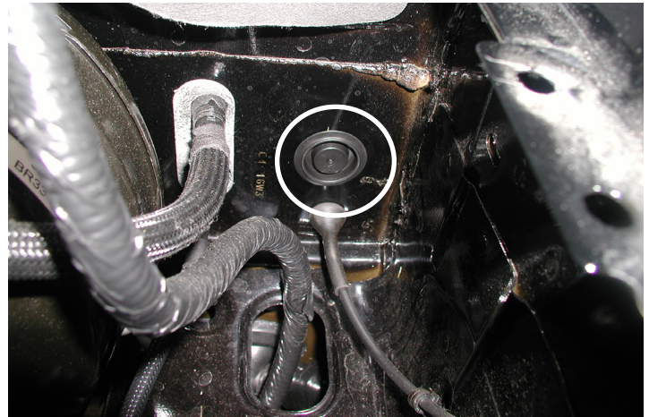
Supplied Grommet Installed
