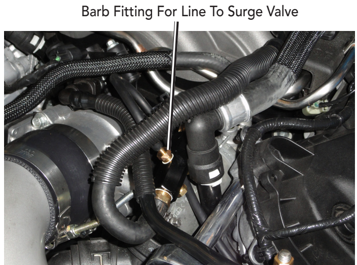
Vacuum Manifold Installed
